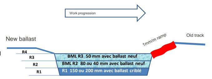
• **Pumping phenomenon in the last 20m** of the ramp on both rails, probably due to a large quantity of screened ballast used and tamped in the connection with the old track. Tamping was performed without « retour chariot » => machine was lifting the old track of a few mm with no consequences on safety;
