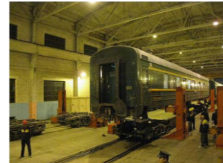
Figure 4-1 Bogie exchange facility Mongolian/Chinese border
