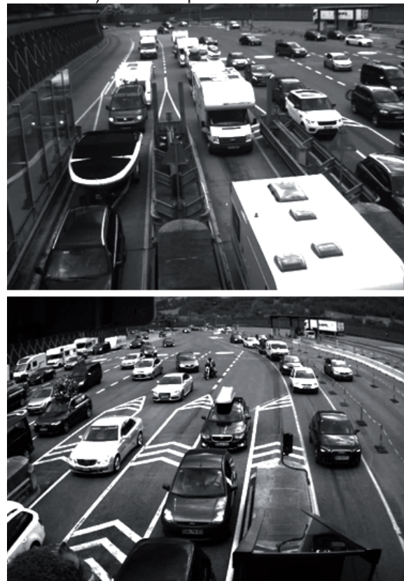
Figure 2: The toll plaza as observed by the cameras. The occupancy on each of the lanes is measured and aggregated. With known camera calibration, a very good estimate of the length of vehicle queues can be measured
